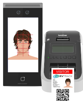
Step 05 On Approval by the Host, the visitors face is added temporarily to the access control face biometric reader & a visitor badge is printed.
